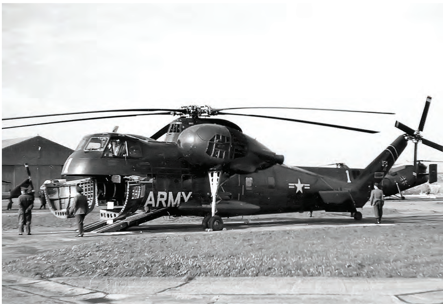
With 4,200 h.p. of lift and a front loading ramp, the CH-37 was a major step forward in the Army's ability to move light vehicles, firepower, and supplies around the battlefield. (U.S. Army photo).
