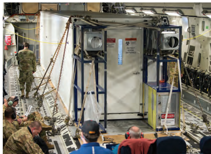
In-flight testing is conducted to certify a Negatively Pressurized Conex prototype at Joint Base Charleston, S.C., April 30, 2020. (U.S. Air Force photo by Staff Sgt. Chris Drzazgowski).
